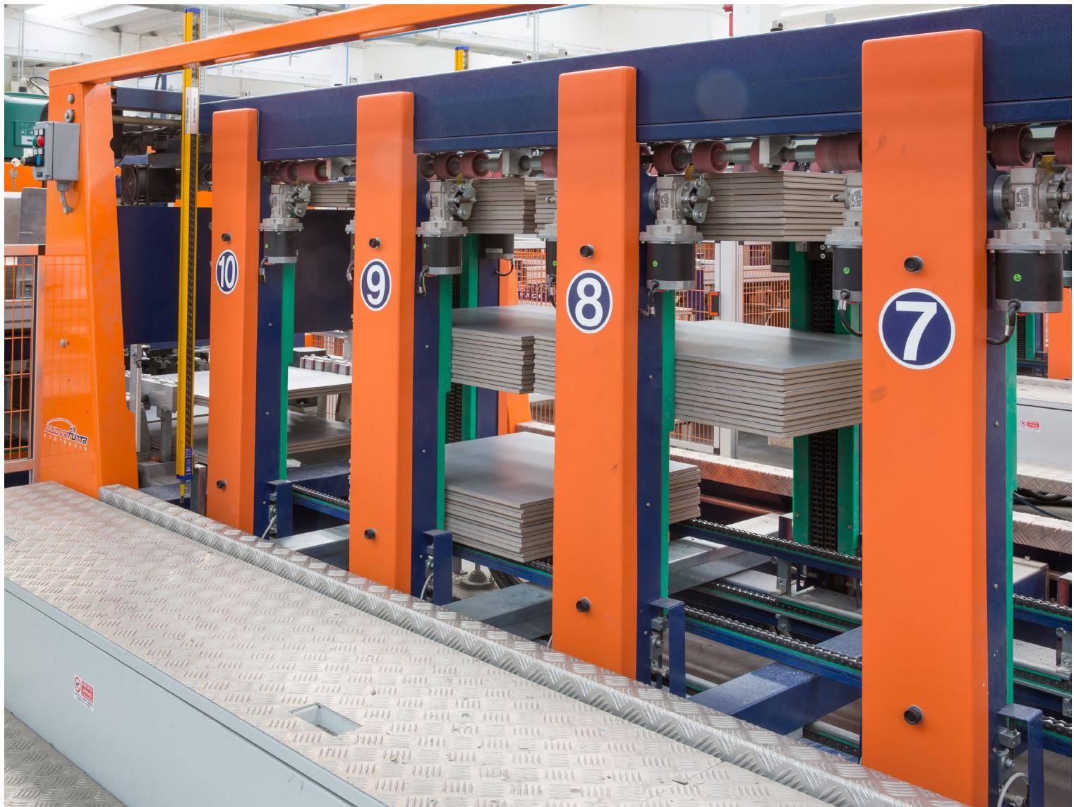
Once the stacks of tiles have been formed, the transfer unit consisting of two timed chains transfers them to the packaging machine.
